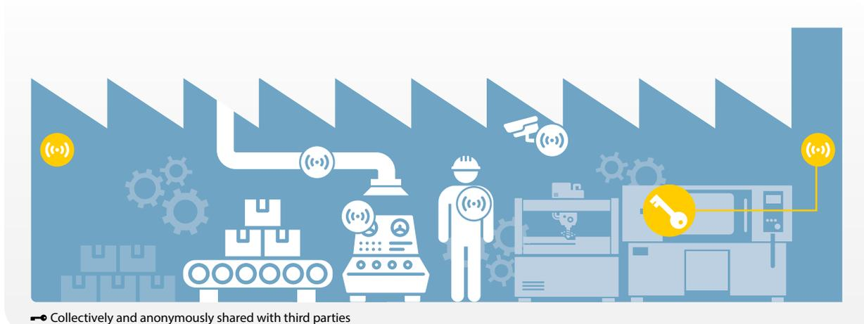
Stationary sensors are carefully distributed throughout the work environment. The concentration of a chemical substance is continuously measured. Modelling tools are used to draw a substance concentration map of the area, making high-concentration zones visible; this allows the location of a source to be identified.
