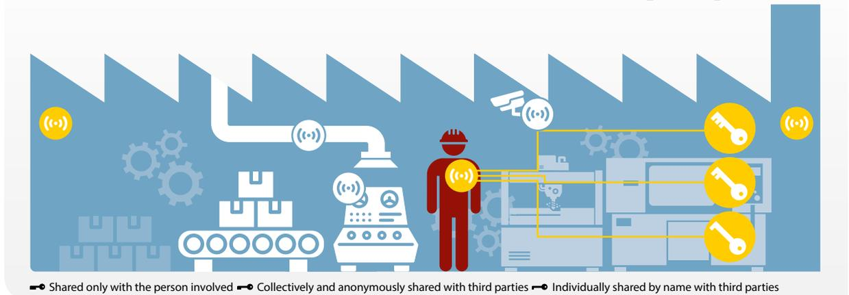
Stationary exposure sensors and modelling tools can be used to draw up concentration maps of workspaces. This can be done for more than one chemical substance simultaneously. If employees are fitted with an ILT device, individual exposure profiles can be developed by combining an individual's indoor location data with the concentration map data.
