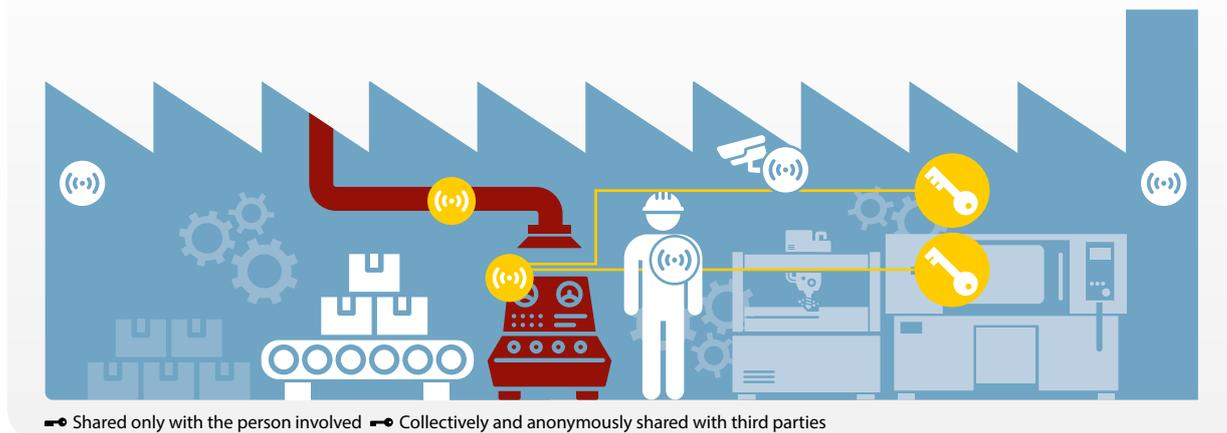
Sensors can be used to monitor the effectiveness of control measures or working procedures. This applies both to sensors measuring chemical substances and to so-called ‘smart sensors’ that measure physical quantities such as temperature, distance, orientation, vibration, pressure, etc. They are not applied to people but to equipment and machinery such as fume extractors. Examples would include:
