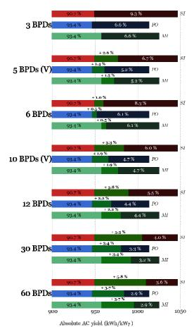
Figure 9: TMY AC yield results for SI(+), PO and MI systems. Shading index values and potential benefits when increasing the amount of BPDs per module in a stepwise fashion from 3 to 60 are illustrated
