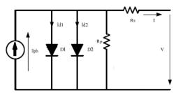
Figure 5: Double diode equivalent circuit for a PV cell
