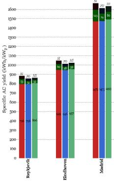
Figure 10: Specific AC yield results for SI(+), PO and MI systems placed in Reykjavik, Eindhoven and Madrid. The red, blue and light-green bars and the corresponding black text indicate the 3-BPD reference specific AC yield in kWh/kWp. The dark green bars and the corresponding white text indicate the potential benefits in kWh/kWp if 60 BPDs per module are used instead of three
