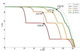
Figure 8: IV responses of example module under partial shading as in Figure 7. The cases of 3, 6, 12 and 60 permodule BPDs are shown. All increases lead to increases in extractable power, as can be seen from the highlighted MPP-values. The grey dashed line represents the IV curve in unshaded conditions. Total irradiance: 1000 W/m2; diffuse irradiance: 200 W/m2; Tmod: 40 °C
