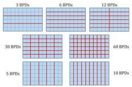
Figure 3: Substring granularities or variation of permodule BPDs investigated in this research. The 3, 6, 12 and 30 BPD cases are referred to as horizontally aligned substrings; the 5 and 10 BPD cases as vertically aligned substrings. Bypass diodes per cell are assumed in the 60 BPD case
