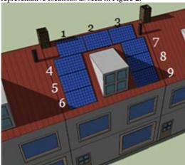
Figure 2: 3D impression of a typical row Dutch house. Dormers, chimneys and poles are usually present, causing obstruction shading to parts of the PV system
