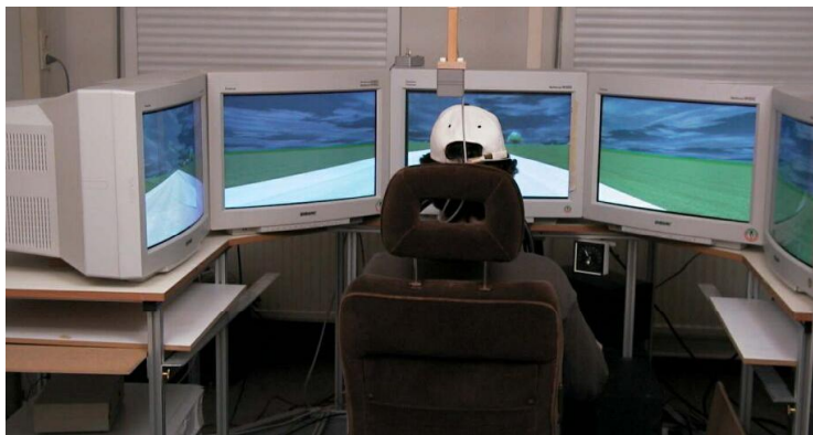
Fig. 4 TNO Low-cost rijnsimulator.
