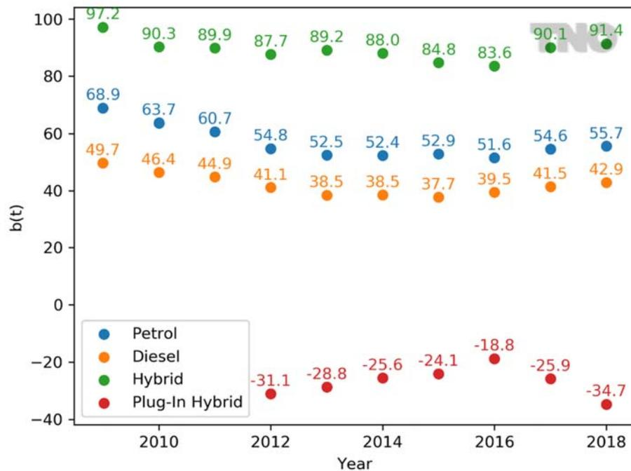
Figure 3: Build Year factor  $b(t)$  for petrol, diesel, and hybrid petrol passenger cars as determined using real world CO<sub>2</sub> values obtained in the Netherlands.
