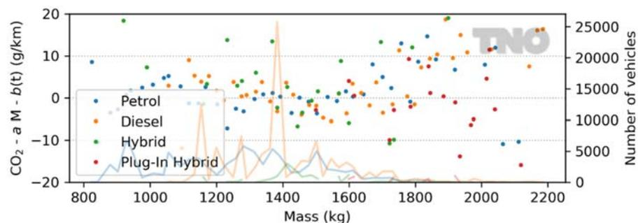
Figure 4: Residual CO<sub>2</sub> dependence ( $CO_2 - aM - b(t)$ ) on mass, of petrol (blue dots), diesel (orange dots), hybrid (green dots), and plug-in hybrid (red dots) vehicles. The number of vehicles is also indicated (lines). Low vehicle numbers, i.e., below 500 are a source of large variations due to limited statistics.
