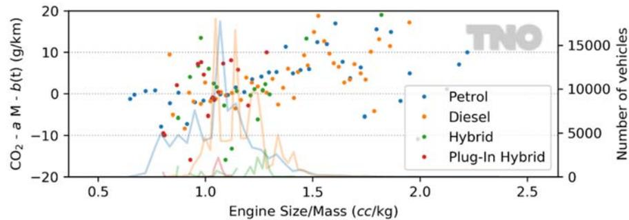
Figure 7: Residual CO<sub>2</sub> dependence ( $CO_2 - aM - b(t)$ ) on **engine size divided by mass**, of petrol (blue), diesel (orange dots), hybrid (green dots), and plug-in hybrid (red dots) vehicles (binned by engine size/mass). The number of vehicles is shown by lines in the corresponding colours.
