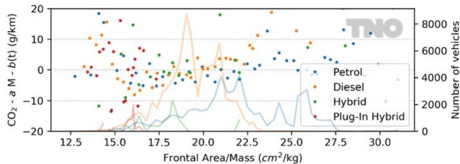
Figure 8: Residual CO<sub>2</sub> dependence ( $CO_2 - aM - b(t)$ ) of petrol (blue), diesel (orange dots), hybrid (green dots), and plug-in hybrid (red dots) vehicles on the **frontal area divided by mass** (binned by frontal area/mass, size of bins shown by lines in the respective colour).
