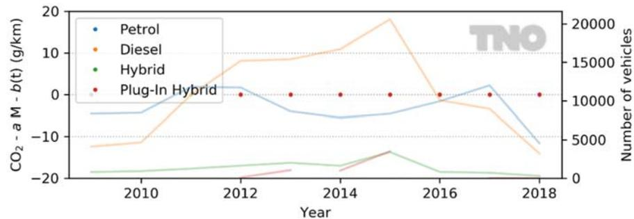
Figure 5: Residual CO<sub>2</sub> dependence ( $CO_2 - aM - b(t)$ ) on **build year**, of petrol, diesel, hybrid, and plug-in hybrid vehicles. This variation is minimal: the dots for each fuel type overlap. The number of vehicles per build year is shown by coloured lines.
