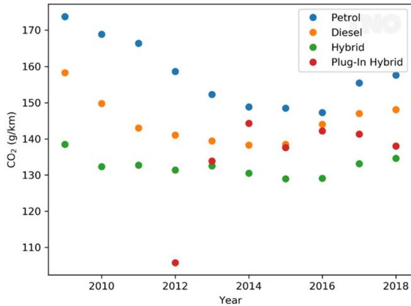
Figure 2: The CO<sub>2</sub> dependence of petrol (blue), diesel (orange), hybrid (green) and plug-in hybrid (red) vehicles in the vehicle subset used for Model M1, on the build year of the vehicle (binned by year). In 2012 the number of plug-in hybrids was very limited.
