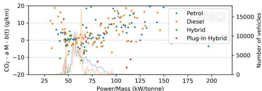
Figure 6: Residual CO<sub>2</sub> dependence ( $CO_2 - aM - b(t)$ ) on **power divided by mass**, of petrol (blue), diesel (orange dots), hybrid (green dots), and plug-in hybrid (red dots) vehicles (binned by power/mass). The number of vehicles in these bins is shown by lines in corresponding colours.
