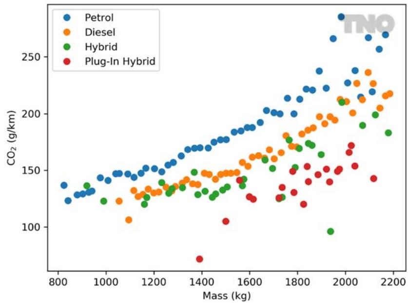
Figure 1: The CO<sub>2</sub> dependence of petrol (blue), diesel (orange), hybrid (green) and plug-in hybrid (red) vehicles in the vehicle subset used for Model M1, on the mass (binned by weight).
