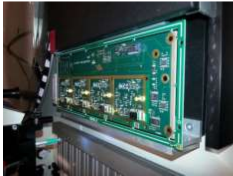
Caption: TNO has developed and built, based on the expertise of the Radar Technology Department, dedicated electronics to control circuits of multiple (transmon) qubits.
