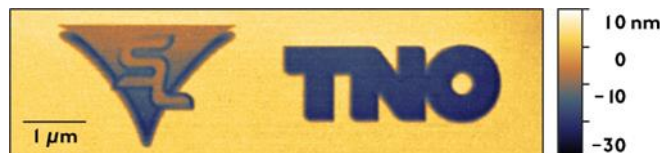
Figure 6: Swiss Litho and TNO logo patterned by the experimental setup shown above.
