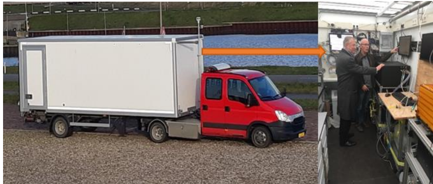
Figure 1. Measurement Van including GHG and aerosol measurement instruments
