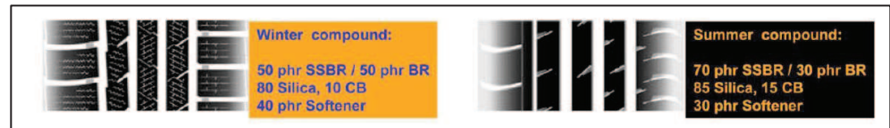
Figure 3.1: Comparison of typical winter and Summer tyre [8].
