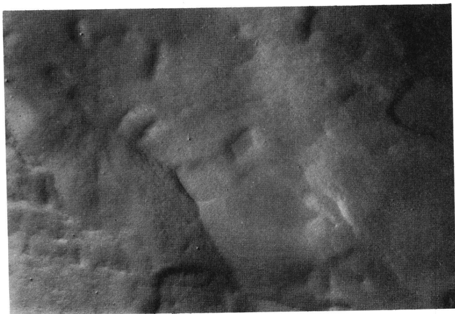
Photo 1. Glucose monohydrate, magnification 8000 x.
