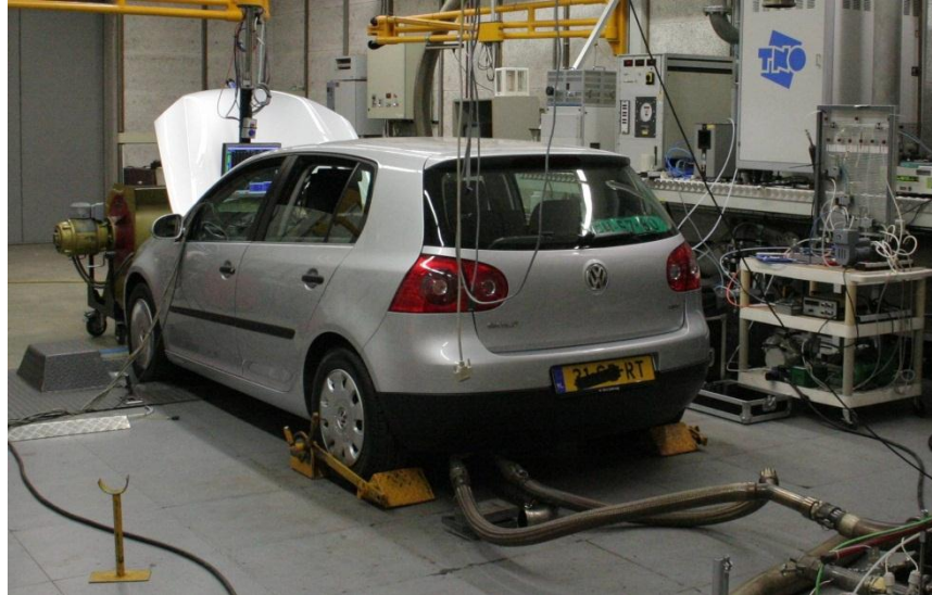
Figure 5: Chassis dynamometer or roller bench
