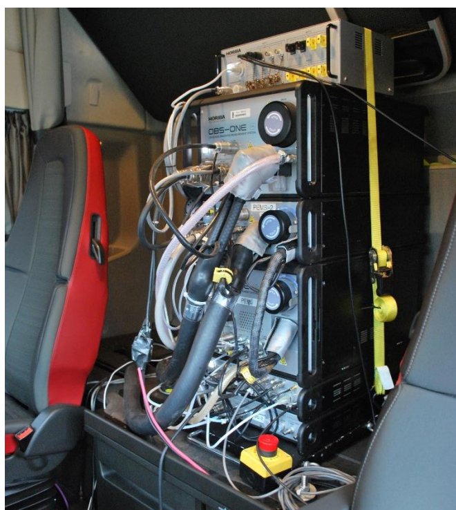
Figure 5 The PEMS analyser mounted in the cabin of the truck.
