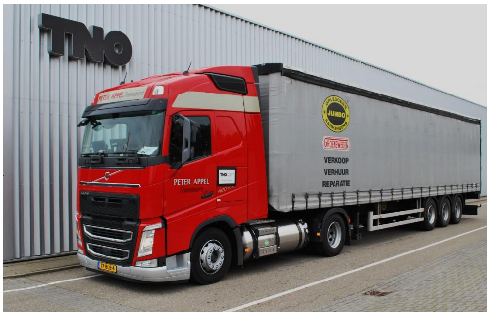
Figure 1 The test subject, a Volvo FH420 tractor with a Euro VI step C certified '1A' dual fuel engine with LNG as the main fuel.
