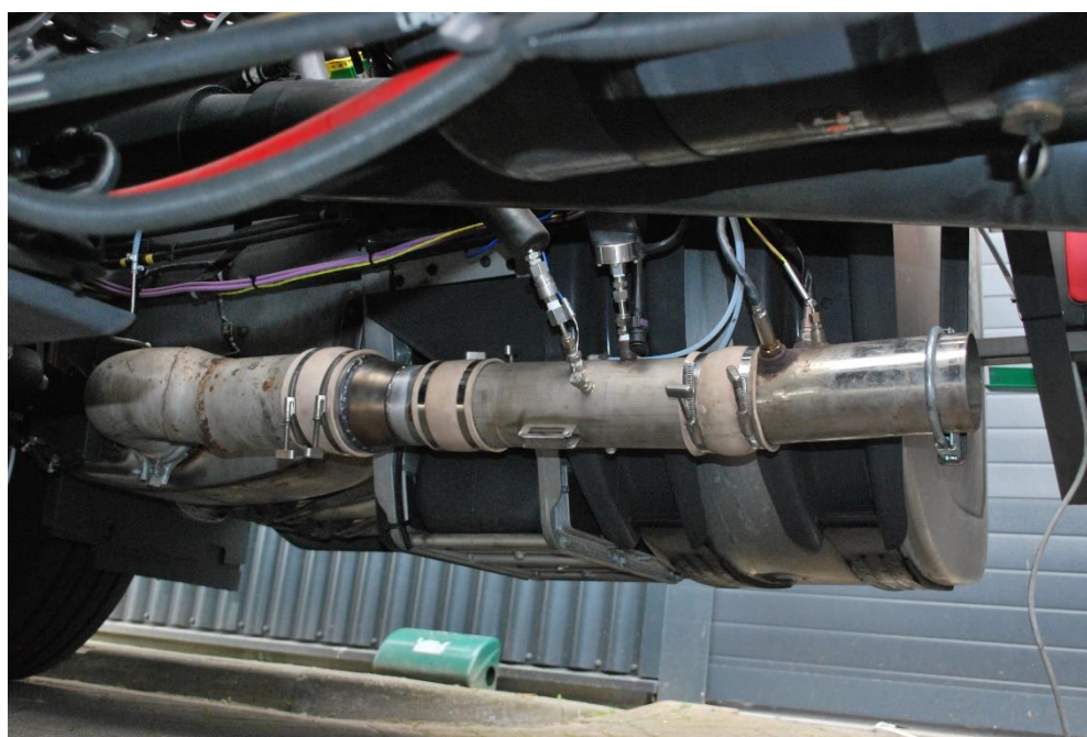
Figure 6 The flow tube connected to the exhaust of the truck.
