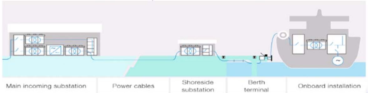
Figure 10: Example shore side infrastructure [14]
