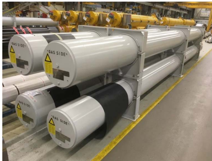
Figure 17: Picture of Constant Pressure Tubes (CPT) as filling system (Linde).
