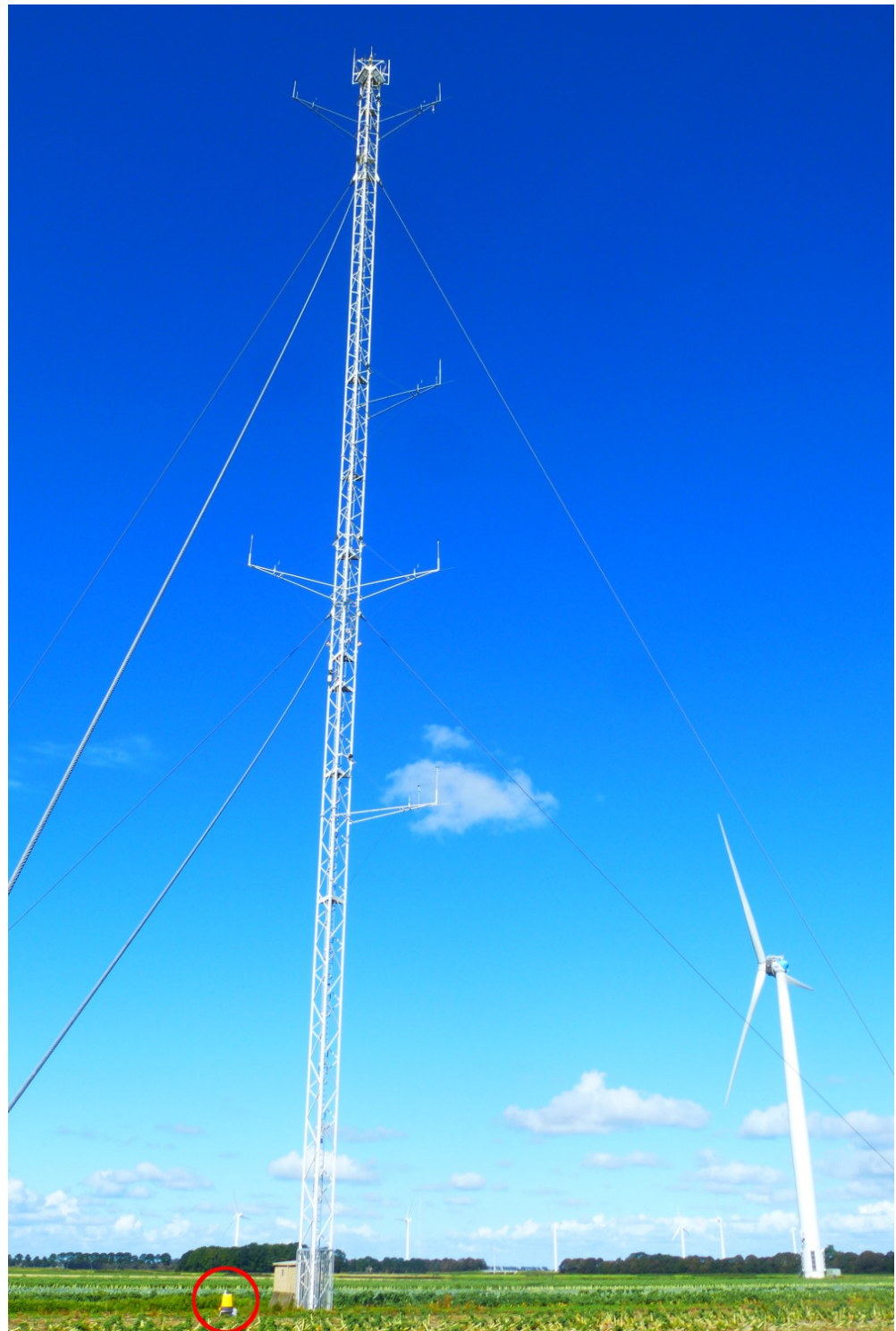
Figure 2: ZephIR 300M, unit 563, indicated in red, at the ECN part of TNO LiDAR Calibration Facility at the base of Meteorological Mast 4
