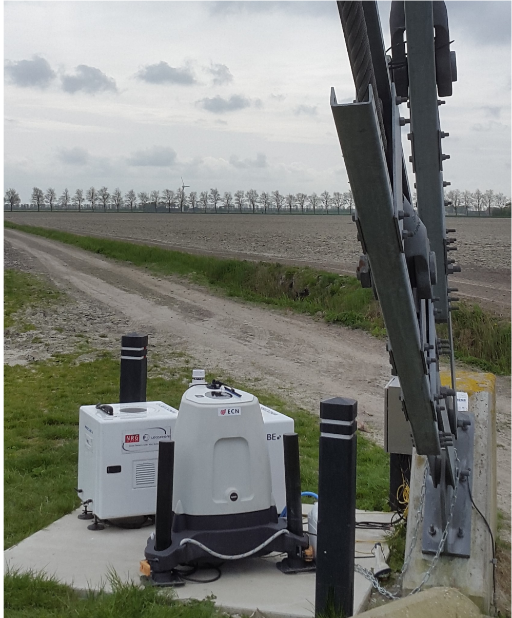
Figure 2: ZephIR 300, unit 315 (front center, labeled ECN ) at the ECN part of TNO LiDAR Calibration Facility next to the guy wire anchor of Meteorological Mast 4
