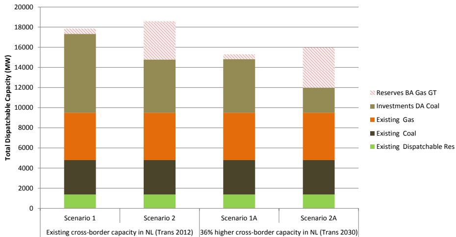
Fig. 7. The total dispatchable capacity in the Netherlands for the residual demand with increasing transmission capacity.
