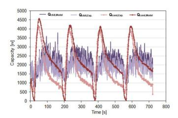
Fig. 8. Comparison between calculated and experimental results for evaporator cooling capacity and condenser capacity.
