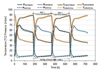
Fig. 6. Experimental and model prediction of pressure and outlet temperature of adsorbent beds.
