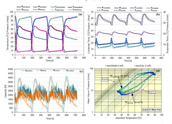
Fig. 11. Comparison between calculated and measured results - 2nd Operation Mode (heat recovery mode): (a) Pressure and outlet temperature profiles of adsorbent beds, (b) Temperature profiles and pressures at condenser and evaporator, (c) Cooling capacity and condenser capacity, (d) Dühring diagram of the Silica gel/water adsorption system at rated conditions.
