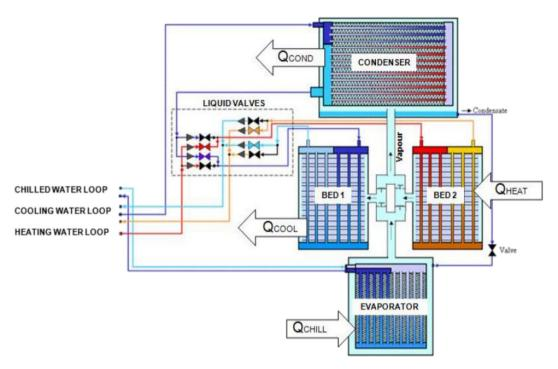
Fig. 1. Schematic diagram of the considered adsorption cooling system, detailed view.
