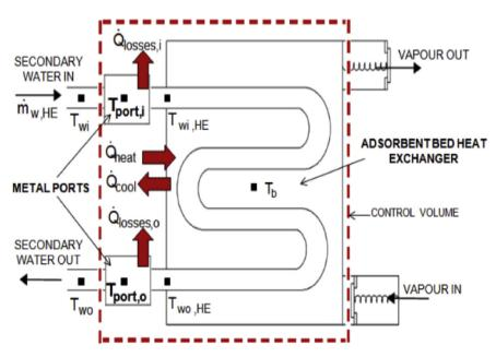
Fig. 4. Single adsorbent bed heat exchanger with the considered control volume (red dashed line). (For interpretation of the references to colour in this figure legend, the reader is referred to the web version of this article.)
