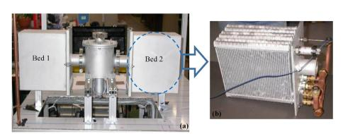
Fig. 2. (a) Two sorption beds connected to the central housing that contains the refrigerant check valves. (b) One sorption bed assembly.
