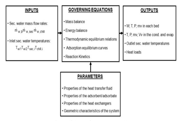
Fig. 5. Simplified structure of the adsorption system model.
