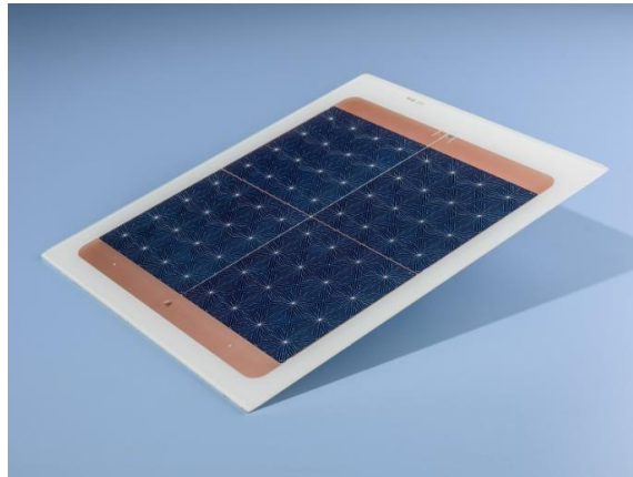
Fig. 3. Picture of a 4 cells mini-module using a CBS without solder mask and with OSP-finish
