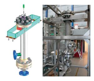
Figure 7. Drawing and picture of the down-scaled membrane module.
