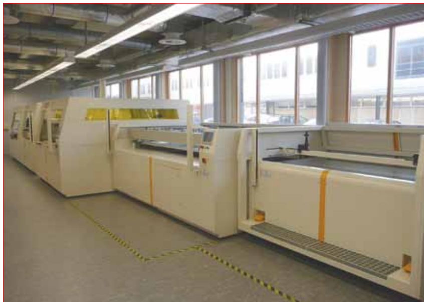
Figure 7. Picture of the pilot line at ECN for manufacturing back-contact modules.
