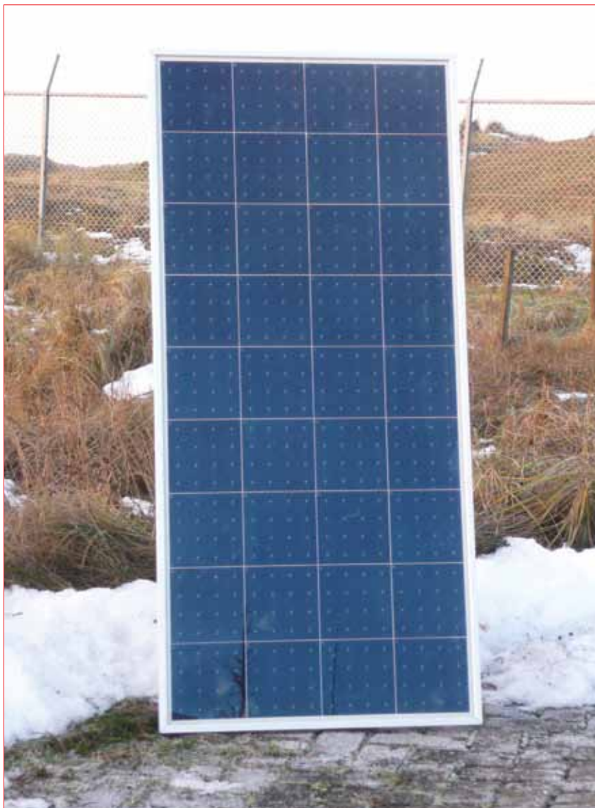
Figure 9. Picture of the finished MWT module. All of the conductive back-sheet is within the active area of the cells. There is no need for bussing at the top and bottom of the module resulting in optimum packing density.
