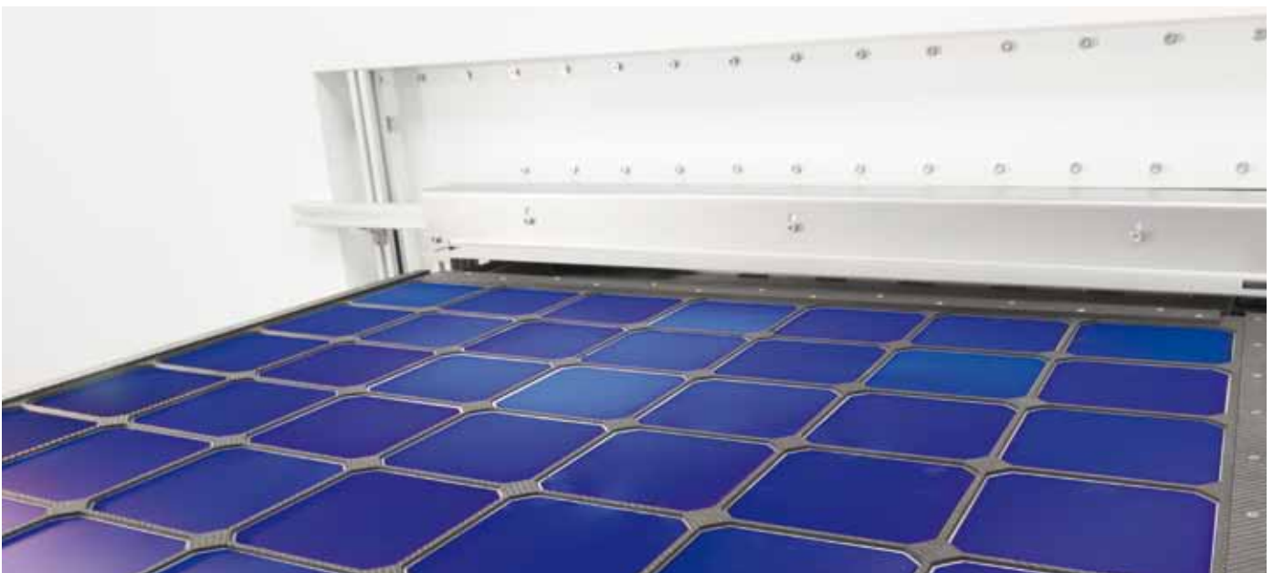
Specialized carriers have been designed by production equipment suppliers, including Meyer Burger, for heterojunction cell production.
