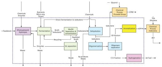
Fig 3: Block diagram of the process developed, including an alternative option with direct fermentation of isobutylene
