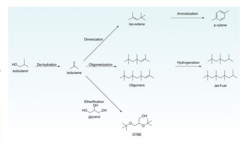
**Fig 2:** Basic chemicals obtained via isobutanol dehydration. Isobutylene market: rubbers and p-Xylene market (e.g. PET)
