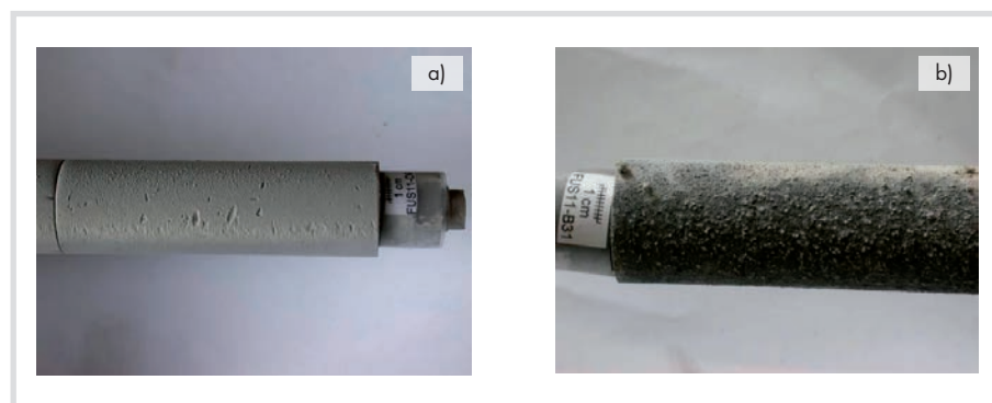
Fig 7. a) deposition test- 42 m; b) deposition test – 38 m; coal/RDF (95/5) scenario.
