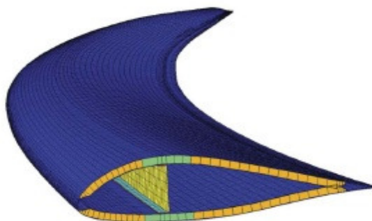
Figure 4. The unidirectional composite fabrics follow the curvature of the blade.
