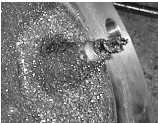
Figure 14. Naphtalene deposit on top flange and spray nozzle of tar scrubber.
