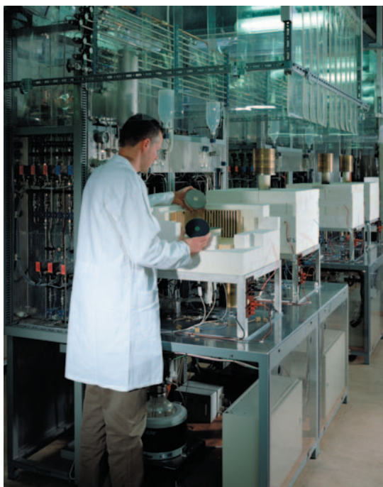
A SOFC-cell is installed by BCT-employee Hans van Wees before testing.
