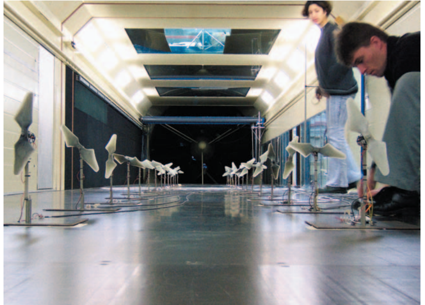
Test system in wind tunnel shows wake effect of wind farms.
