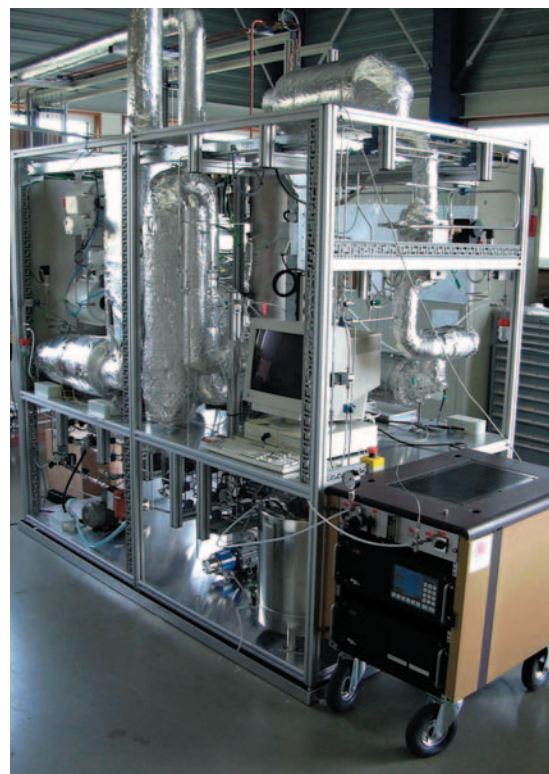
Fuel processor installation for producing hydrogen from bioethanol on a 10 kW scale.
