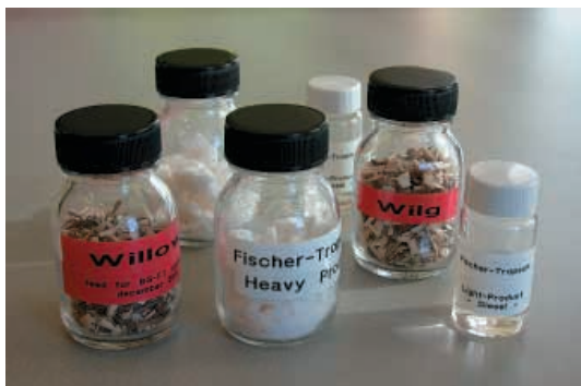
'Green diesel' from biomass and waste produced via the Fischer-Tropsch synthesis.
