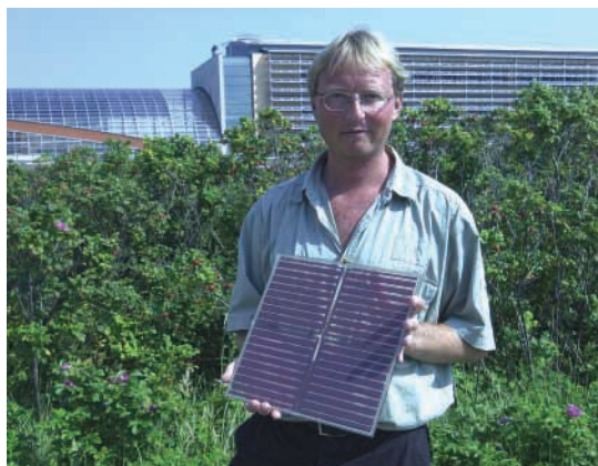
Martin Späth with a prototype of a 30×30 cm 2 dye-sensitised solar module containing 4 integrated cells and fabricated at ECN.
