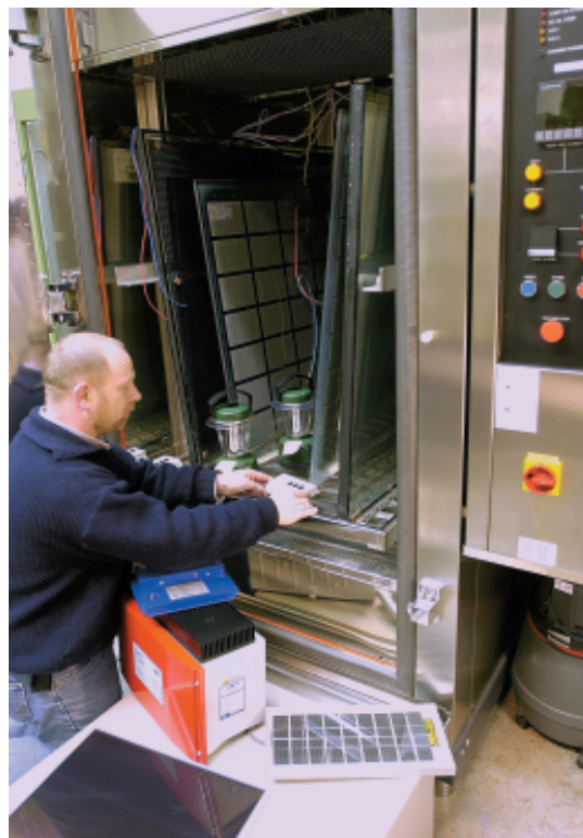
Henk Kisteman loads the climate chamber for testing solar energy components under extreme conditions.
