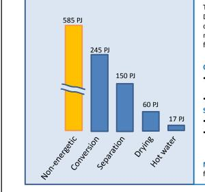
The figures on the left show the distribution of the energy use in the Dutch Process Industry based on the Berenschot study. The energy demand consists mainly of heat for different application. In addition mainly in the petrochemical industry energy carriers are used as feedstock, for example natural gas to produce hydrogen.
