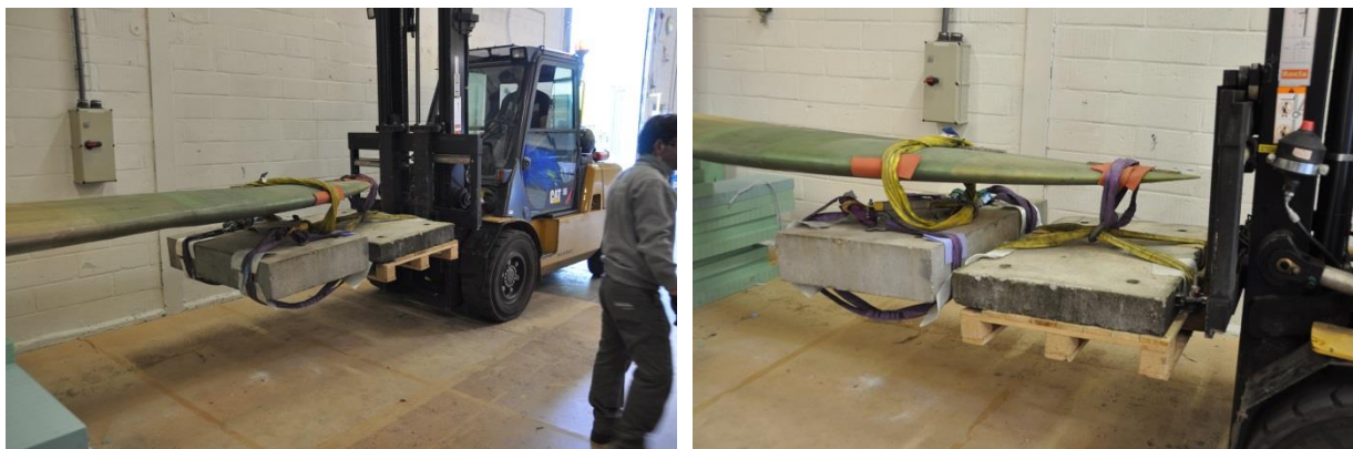
Figure 5-17: Static Extreme load test – Flapwise direction
