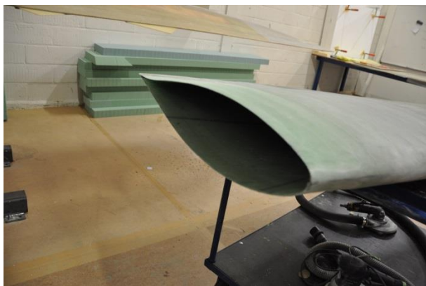
Figure 5-6: Grinded prototype tip for smooth transition
