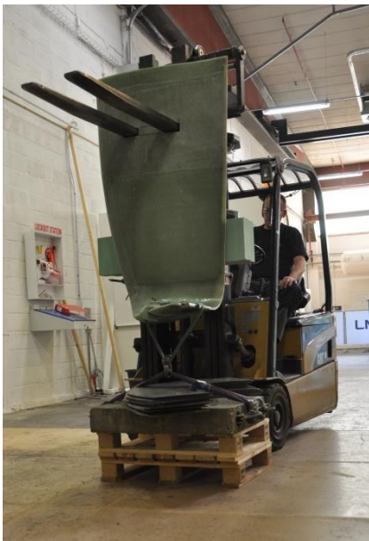
Figure 5-20: Static Extreme load test Winglet – Flapwise direction
