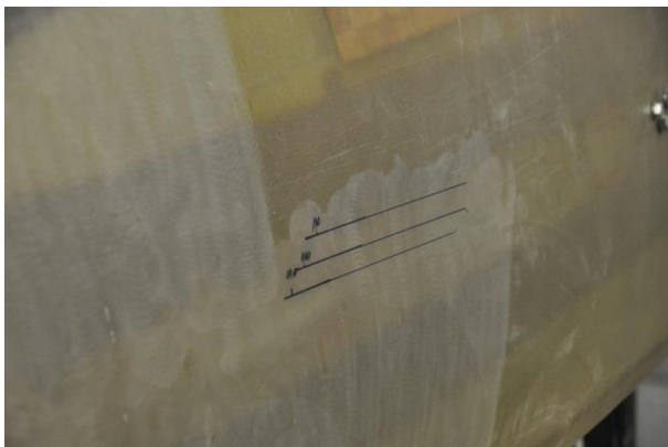
Figure 5-9: Markings on the blade for drain holes and anchor block after grinding
