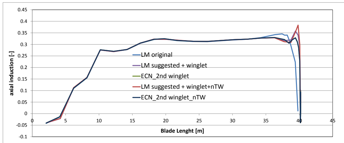
Figure 4-11: Axial induction along the blade
