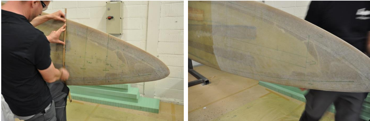
Figure 5-10: Marking blade for alignment and gluing areas
