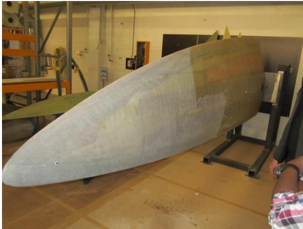
Figure 5-8: Grinded LM38.8P surface and installed distance plugs
