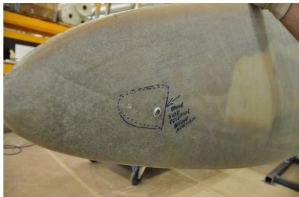
Figure 5-9: Markings on the blade for drain holes and anchor block after grinding
