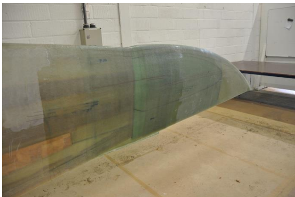
Figure 5-13: Connection after over-lamination process has finalized
