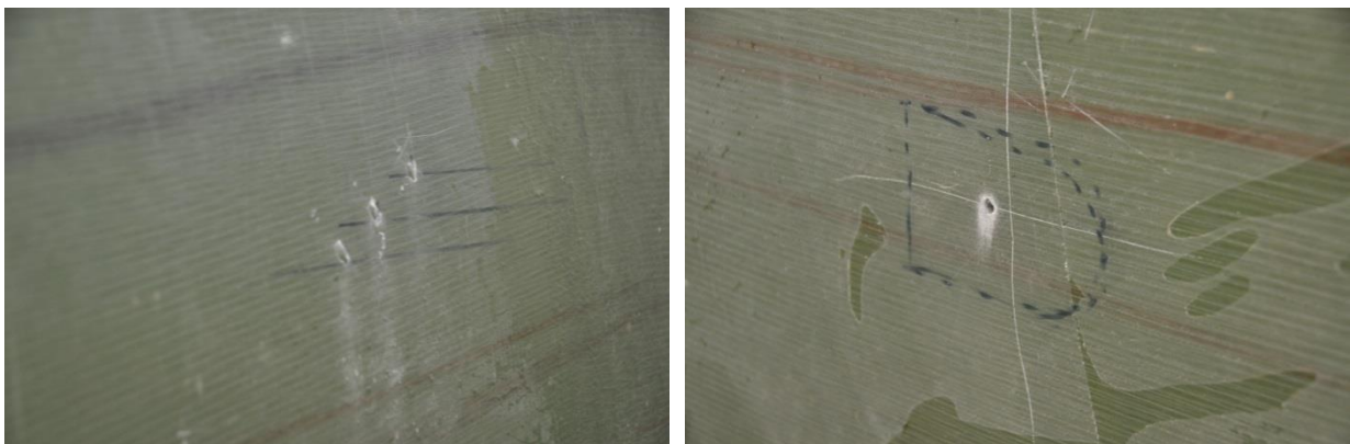
Figure 5-14: Drilled drain holes and receptor hole for extending lightning protection
