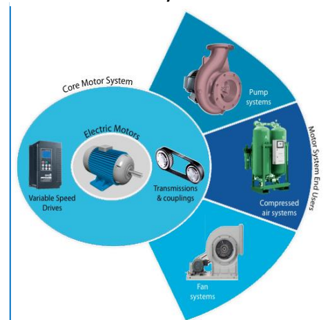
Figure 5: Most common elements of an electric motor driven system
