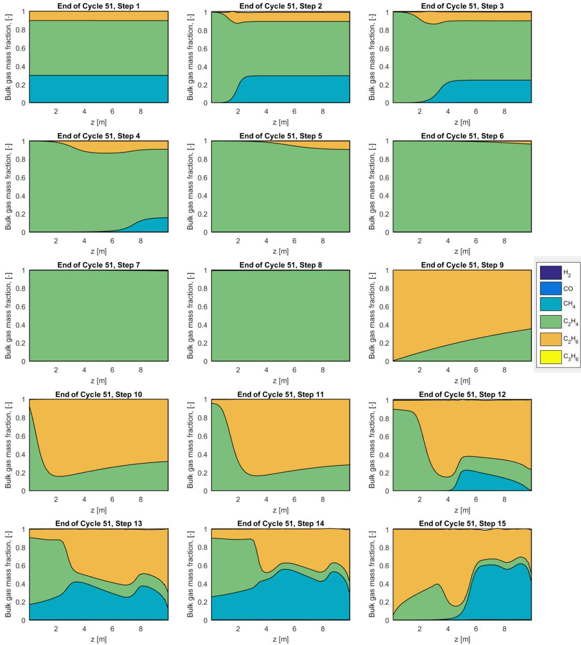
**Figure 23:** Gas phase concentrations vs axial coordinate at the end of each step during OPERA cycle, conditions in **Table 23** (1) Adsorption (2) Rinse (3) Pressure equalisation 1 (4) Pressure equalisation 2 (5) Pressure equalisation 3 (6) Pressure equalisation 4 (7) Pressure equalisation 5 (8) Depressurisation (9) Purge (10) Pressure equalisation 5 (11) Pressure equalisation 4 (12) Pressure equalisation 3 (13) Pressure equalisation 2 (14) Pressure equalisation 1 (15) Repressurisation
