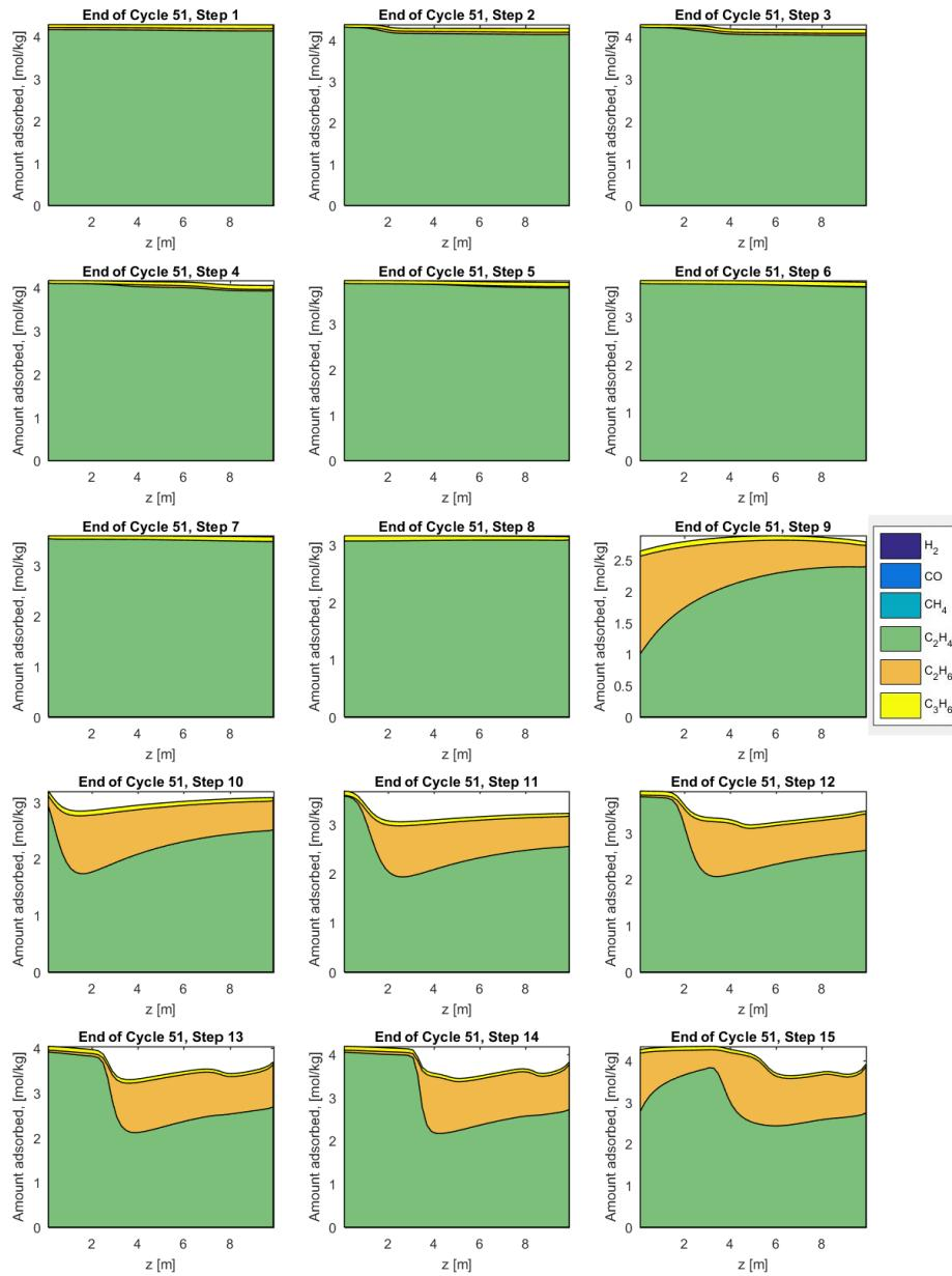
**Figure 25:** Adsorbate loading vs axial coordinate at the end of each step during OPERA cycle, conditions in **Table 23** (1) Adsorption (2) Rinse (3) Pressure equalisation 1 (4) Pressure equalisation 2 (5) Pressure equalisation 3 (6) Pressure equalisation 4 (7) Pressure equalisation 5 (8) Depressurisation (9) Purge (10) Pressure equalisation 5 (11) Pressure equalisation 4 (12) Pressure equalisation 3 (13) Pressure equalisation 2 (14) Pressure equalisation 1 (15) Repressurisation
