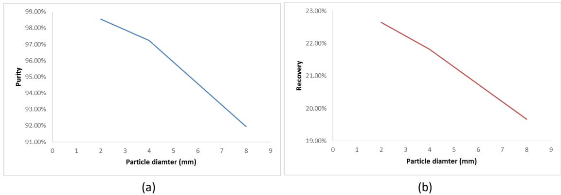
**Figure 13:** Effect of Particle size on bed performance (a) Product purity. (b) Product recovery
