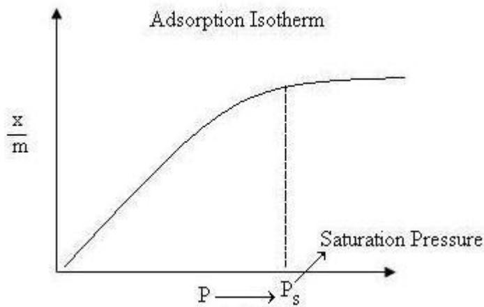
**Figure 3:** Basic Adsorption Isotherm [3]
