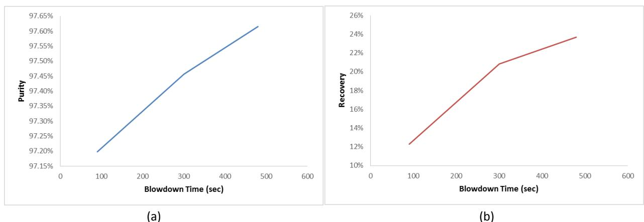
**Figure 18:** Effect of Blowdown time on bed performance (a) Product purity. (b) Product recovery
