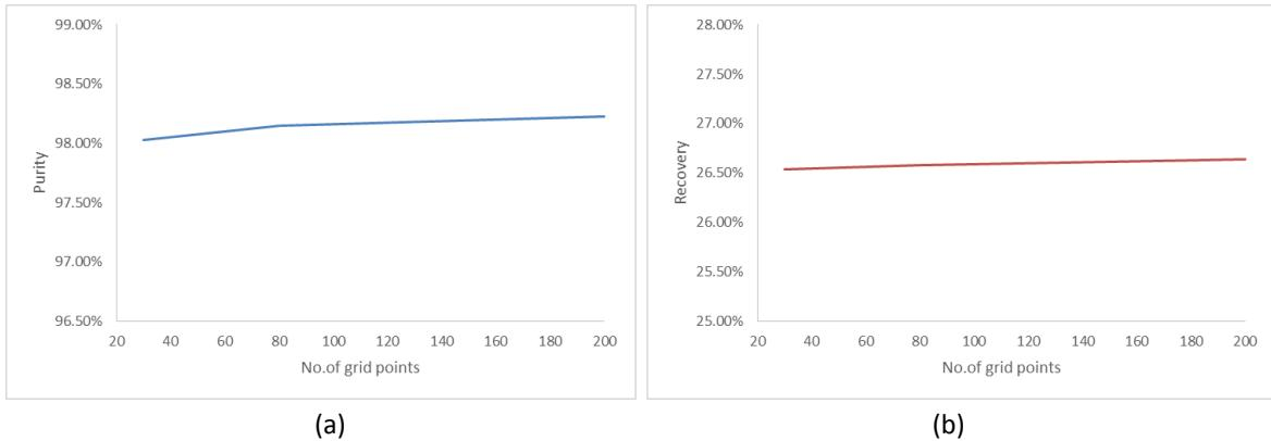
**Figure 20:** Effect of Grid points on bed performance (a) Product purity. (b) Product recovery
