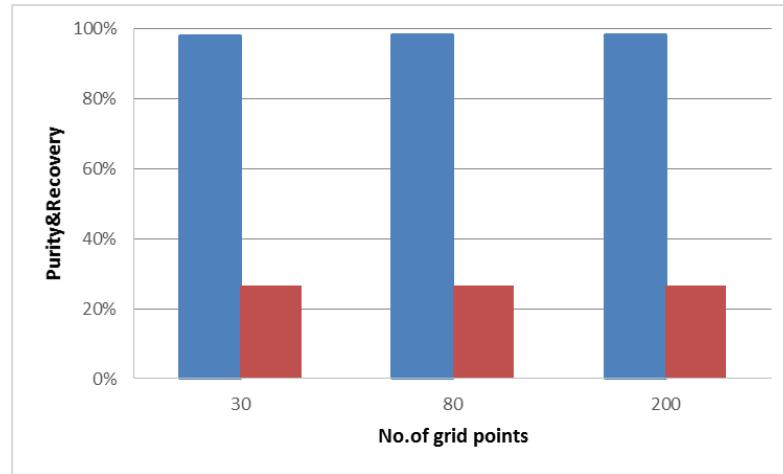
**Figure 9:** Effect of grid points on bed performance
