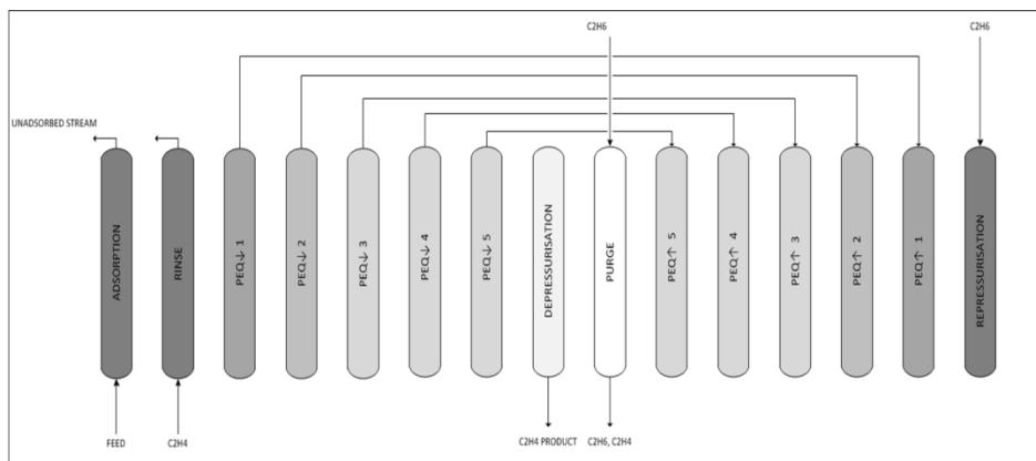
**Figure 8:** 15 step OPERA cycle
