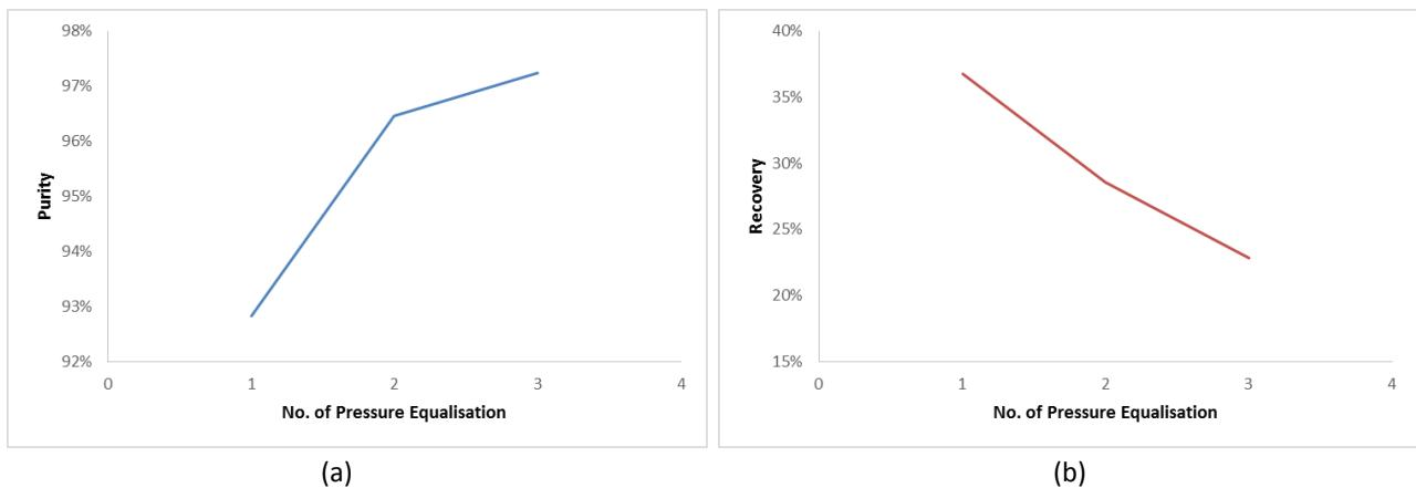
**Figure 15:** : Effect of Number of Pressure Equalisations on bed performance (a) Product purity. (b) Product recovery
