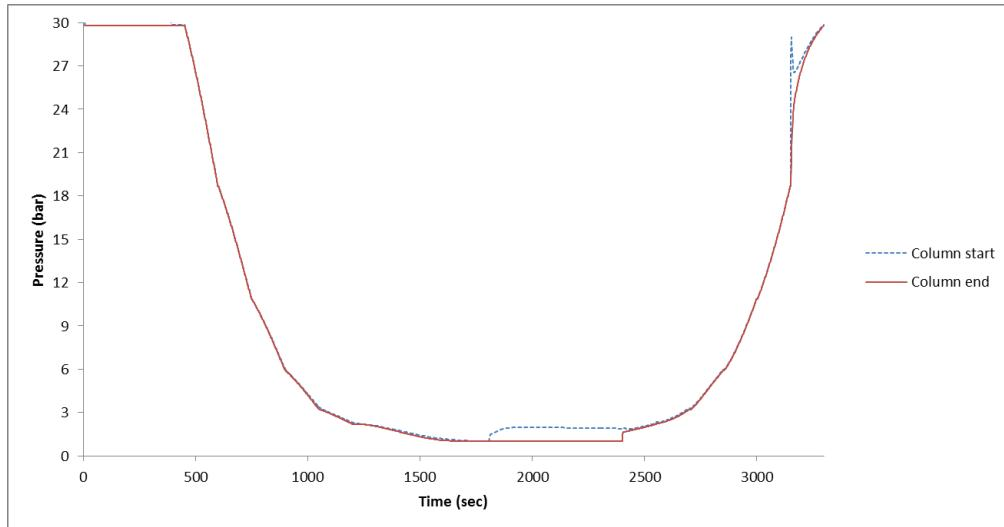
**Figure 10:** Column pressure development over the 15 step OPERA cycle
