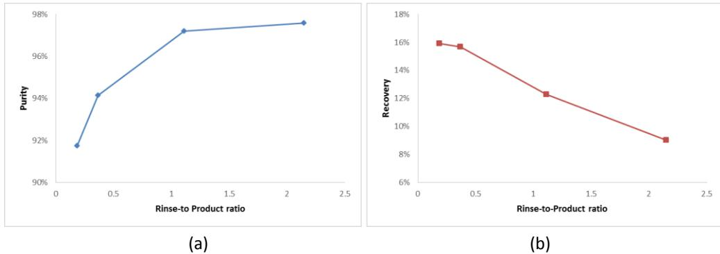
**Figure 11:** Effect of rinse-to-product ratio on bed performance (a) Product purity. (b) Product recovery
