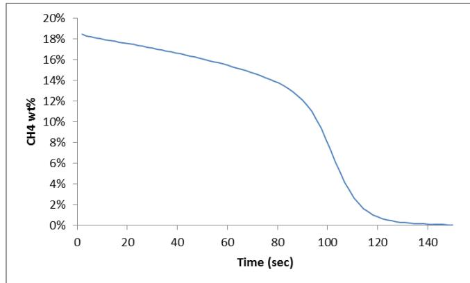
**Figure 17:** Effect of Pressure Equalisation time on CH<sub>4</sub> % in the bed
