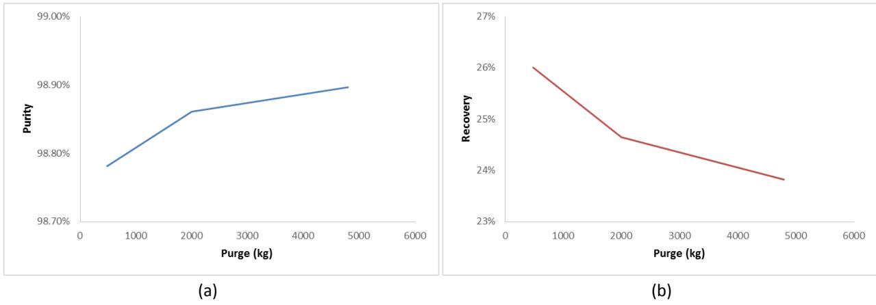
**Figure 12:** Effect of Purge amount on bed performance (a) Product purity. (b) Product recovery
