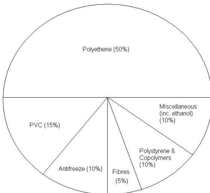
Figure 1: Uses of ethylene/proportions of synthetic organic chemicals which are made from ethylene [13]
