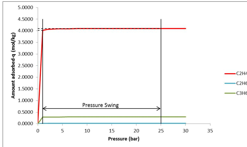
**Figure 5:** Adsorption Isotherm for stream composition before  $C_2$  splitter
