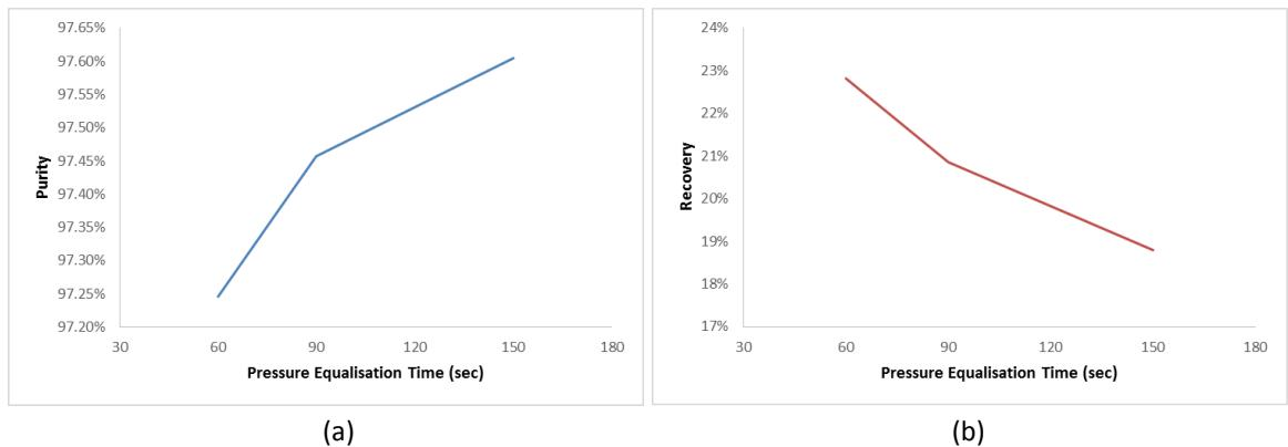
**Figure 16:** : Effect of Pressure Equalisation time on bed performance (a) Product purity. (b) Product recovery
