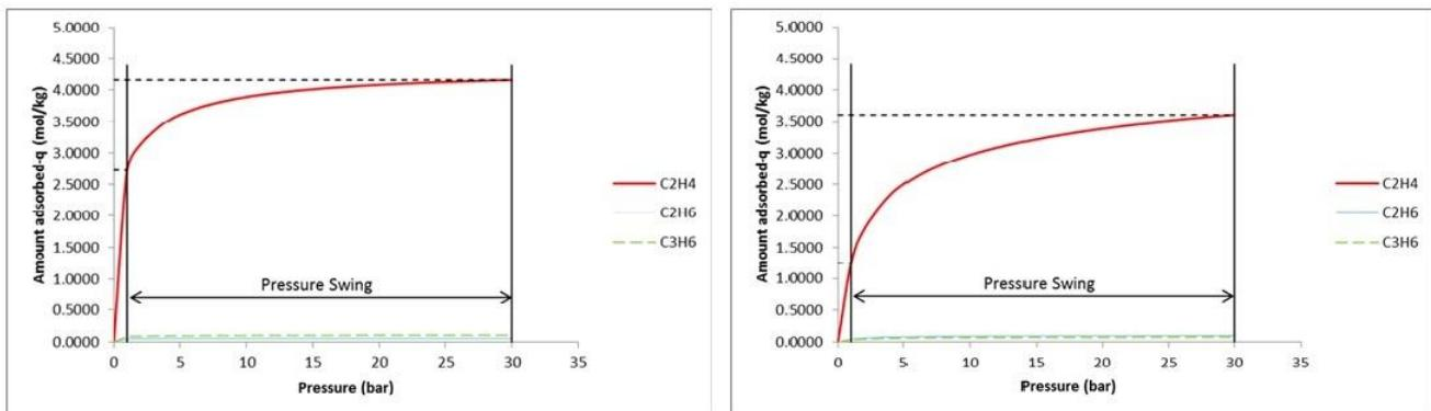
**Figure 6:** Adsorption Isotherm variation with Temperature
