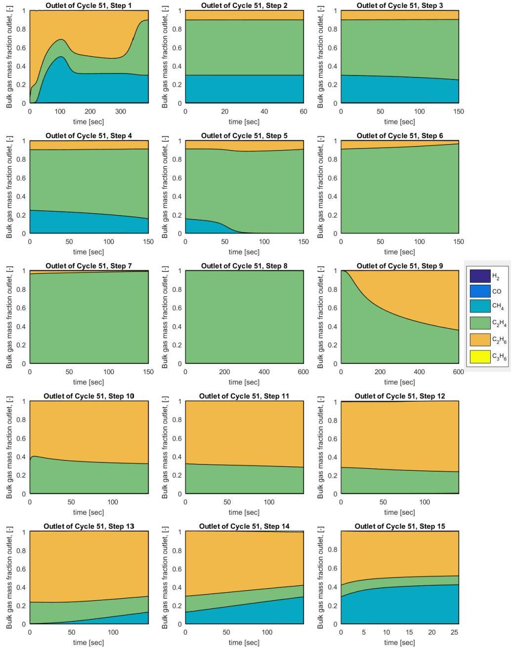
**Figure 24:** Outlet gas phase concentration vs time variation for each step of OPERA cycle, conditions in **Table 23** (1) Adsorption (2) Rinse (3) Pressure equalisation 1 (4) Pressure equalisation 2 (5) Pressure equalisation 3 (6) Pressure equalisation 4 (7) Pressure equalisation 5 (8) Depressurisation (9) Purge (10) Pressure equalisation 5 (11) Pressure equalisation 4 (12) Pressure equalisation 3 (13) Pressure equalisation 2 (14) Pressure equalisation 1 (15) Repressurisation
