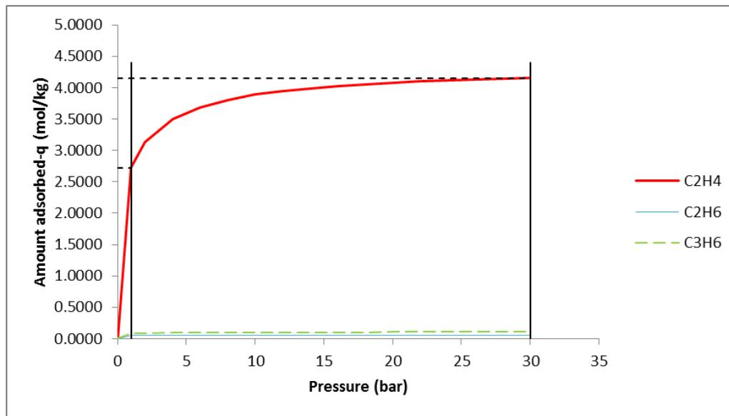
**Figure 4:** Adsorption Isotherm for stream composition after Acetylene ( $C_2H_2$ ) converter
