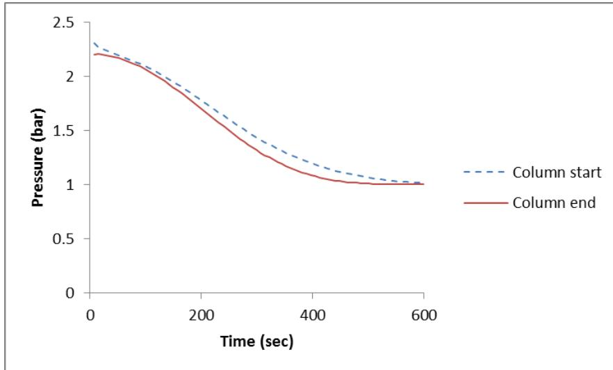
**Figure 19:** Pressure drop profile at the start and end of the column during the blowdown step
