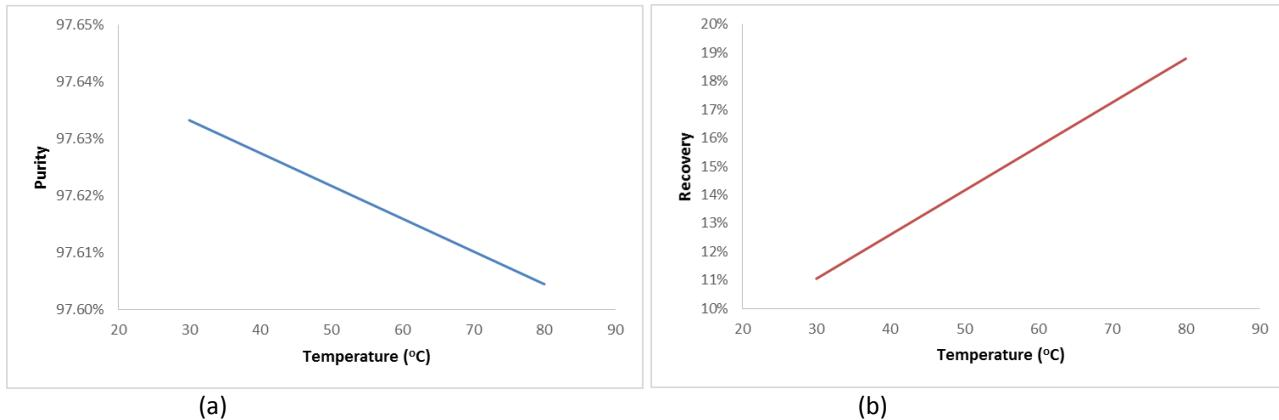
**Figure 21:** Effect of temperature variation on bed performance (a) Product purity. (b) Product recovery
