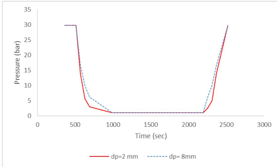
**Figure 14:** Pressure variation along the cycle with varied particle size
