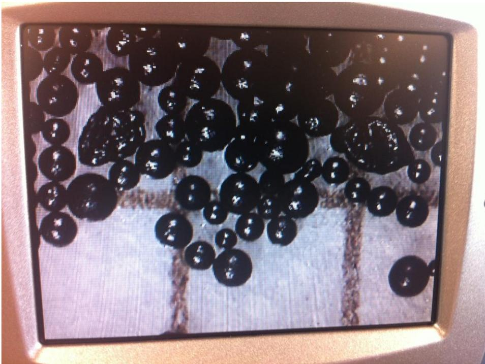
**Figure 20:** BrightBlack adsorbent, photo was made with a microscope with 2.5 times magnification; squares have a size of 1x1 mm
