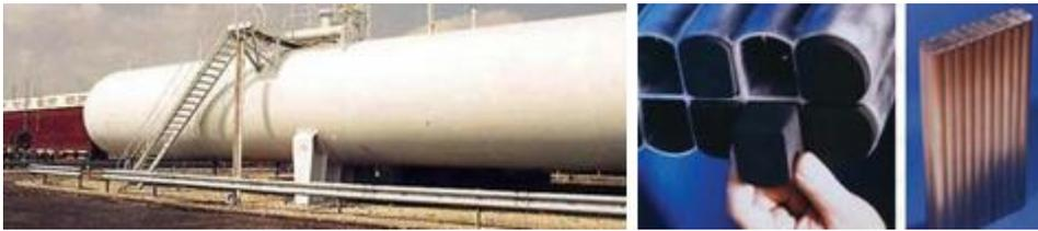
Figure 6: ANG (a) diurnal storage, (b) for vehicular application (GL industrial services)
