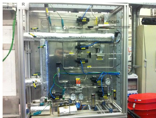
**Figure 15:** Photo of the controllerboard, the arrows mark the different flowmeters/controller and the direction of the flow
