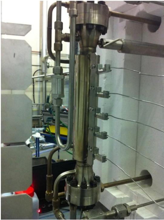
**Figure 17:** The reactor of the hystore apparatus
