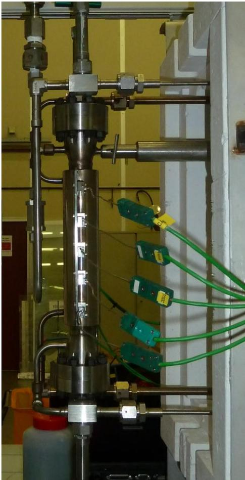
**Figure 16:** Photo of one side of the reactor, here 5 thermocouples can be seen which measurement is influenced by the temperature of the reactor wall. The other side is slightly mirrored, because there is a small deviation in the height of the thermocouples.
