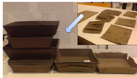
Figure 6: Examples of containers obtained from agricultural by-products by compression-moulding
