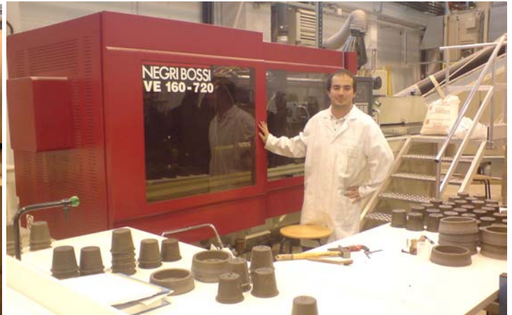
Figure 4: William, technical officer in Agromat, producing flower pots by injection-moulding
