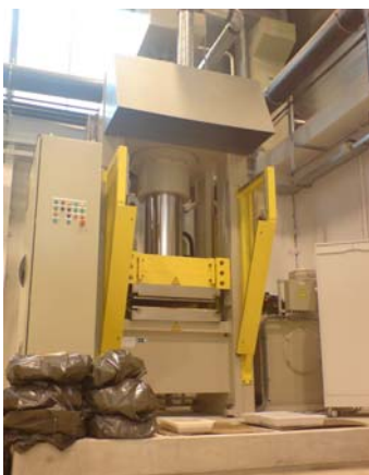
Figure 5: The Agromat 400 tonnes hot press used to make 100% natural composites
