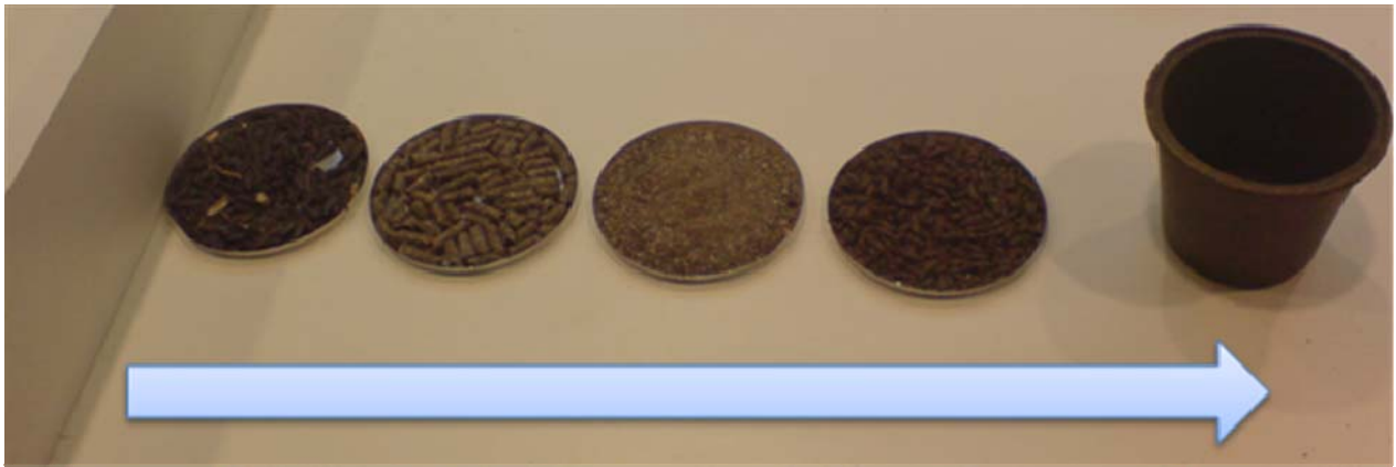
Figure 3: An example of application, from the sunflower seeds to the planting out flower pot going through all intermediate steps: sunflower oil cake, crushed oil cake, extruded and plasticized pellets
