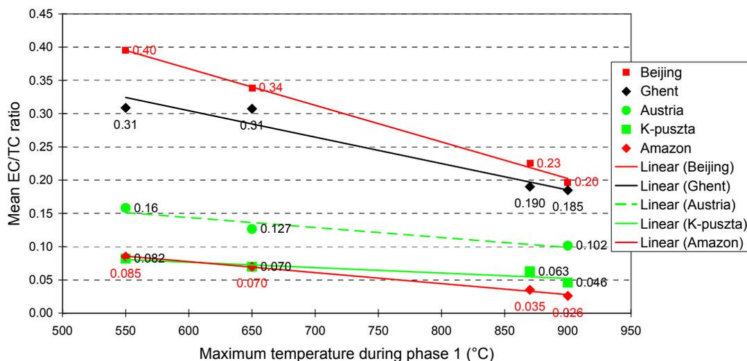
Figure 2. Average EC/TC ratio as a function of maximum temperature in the first phase (in pure He) of the analysis protocol. The average EC/TC ratios are indicated by the symbols and are also given in numeric form. The four analysis protocols from left to right are A3, E2, N2 and ST. All data were obtained with our instrument B.
