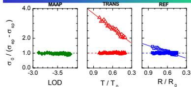
Correction functions for filter loading effects, determined from pure combustion particles; reference absorption coefficient is  $\sigma_{ap} = \sigma_{ep} - \sigma_{sp}$ .
