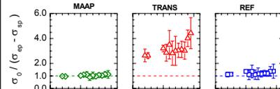
Correction functions for the effect of aerosol light scattering, determined from kerosene soot - ammonium sulphate mixtures
