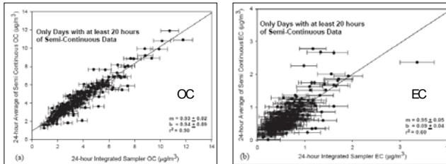
Fig. 5. Comparison of 24-h average semi-continuous analyzer and daily integrated sampler fine particle organic and elemental carbon at the St. Louis-Midwest SuperSite for the year 2002 data set: (a) organic carbon; and (b) elemental carbon. The available hourly concentrations measured by the semi-continuous instruments for days with less than 24 valid measurements are used to estimate the 24-h average.
