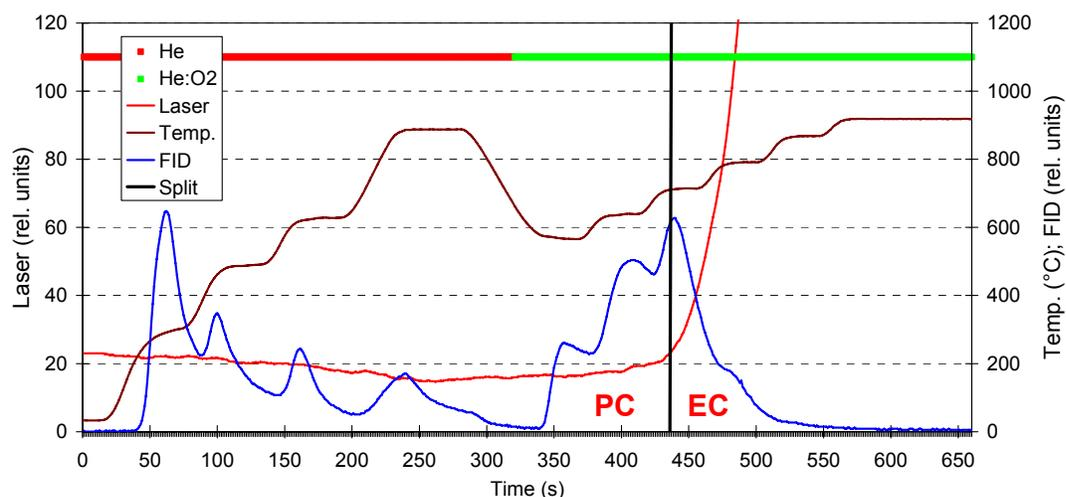
Figure 1. TOT thermogram, obtained with an instrument from Sunset Laboratory and the NIOSH temperature protocol, for an urban PM<sub>2.5</sub> quartz fibre filter sample collected at Ghent.
