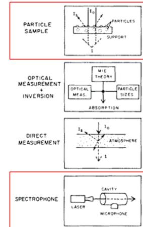
Sketches of the major categories of measuring light absorption by aerosol particles, the graph is taken from the Proceedings of the First International Workshop on Light Absorption by Aerosol Particles
