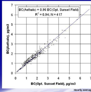
Optical BC measurements delivered by the Sunset Field instrument are consistent with Aethalometer data
