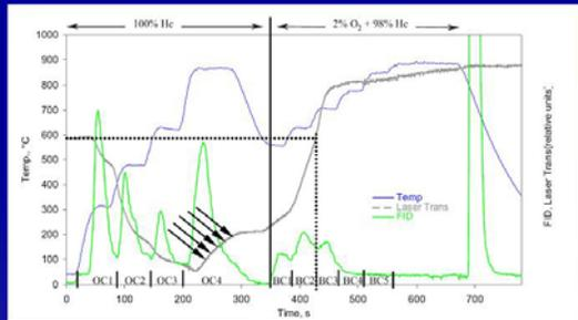
Thermo-optical method with last step at 870°C
