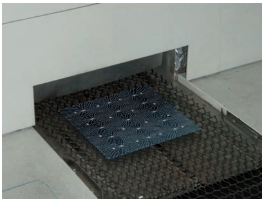
The first Pin-Up cell with a silicon nitride coating on both sides.
