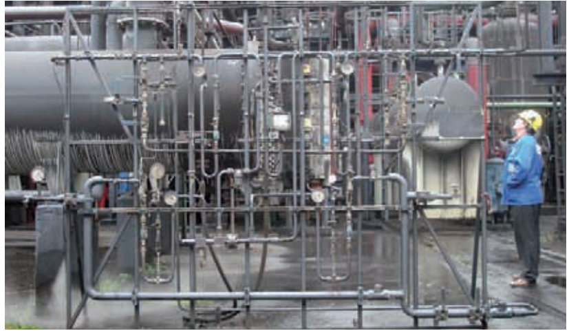
Membrane test installation for ammonia separation in Tertre (BE).
