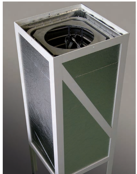
Compact heat storage as being built. Plates and cover have to be finished.
