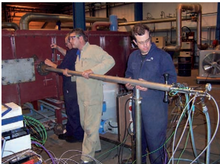
Deposition probe mounted in exhaust pipe.
