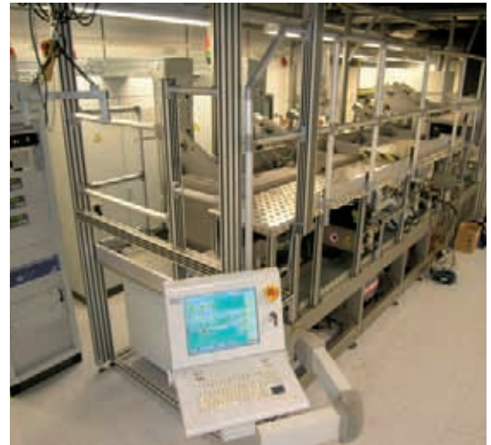
Picture left and below: Prototype plasma deposition machine for producing thin film silicon solar cells on foil.
