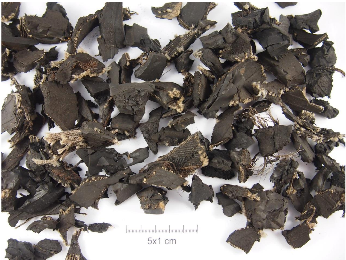
Figure 1: METRECO - photograph of the final product received at ECN for physical/chemical analyses and combustion testing.
