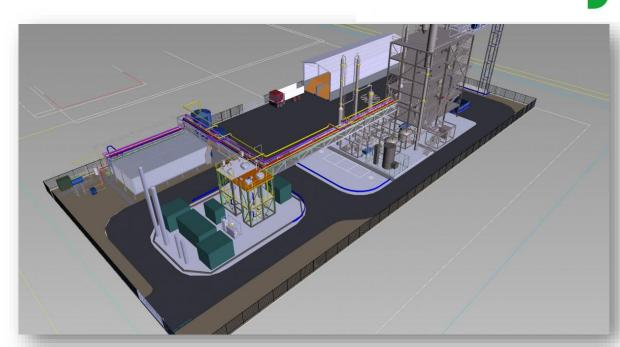
MILENA indirect gasification + OLGA tar removal system + ESME methanation = improved efficiency to bio-SNG
