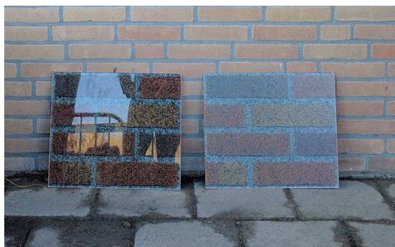
Figure 4: Panels with a brick design coverage of 45% with flat front glass on the left and structured front glass on the right.
