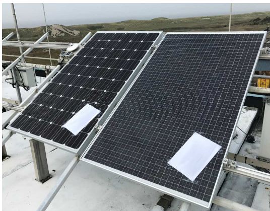
Figure 8: Outdoor setup with on the left a standard module and on the right the Tessera ® module
