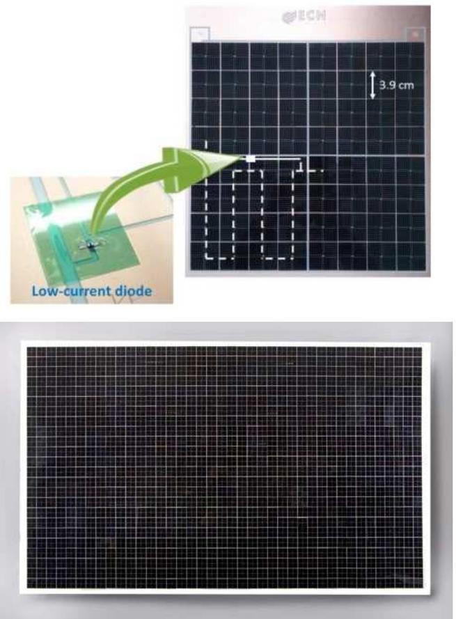
Figure 1a: A building block of the TESSERA concept consisting of 64 mini cells connected in series and protected by 4 low current in laminate diodes; 1b: a full size TESSERA module.
