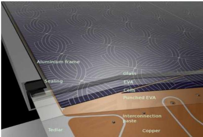
Figure 2: Presentation of the build-up of a MWT back contact module using an interconnecting backsheet.
