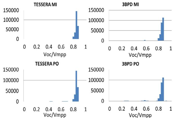
Figure 6. Vmpp/Voc for a 3BPD module with micro-inverter or power optimizer and a TESSERA module with micro-inverter or power optimizer
