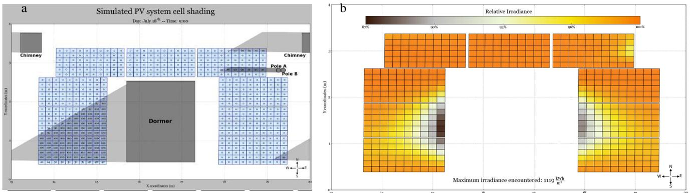
Figure 4. a. Placement of modules on a typical Dutch roof including a dormer, chimney and exhaust poles, b. Effective irradiance reaching the modules in a typical meteorological year for NL.
