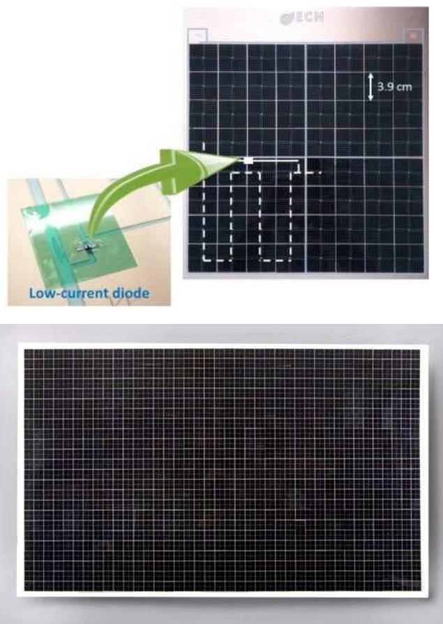
Figure 1a: A building block of the TESSERA concept consisting of 64 mini cells connected in series and protected by 4 low current in laminate diodes; 1b: a full size TESSERA module.
