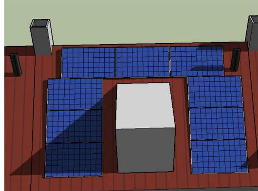
Figure 3. System layout for the yearly yield calculations. A typical Dutch roof including a dormer, chimney and exhaust poles,
