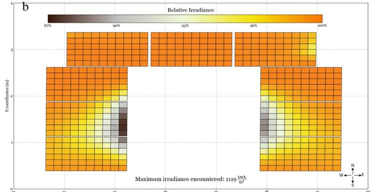
Figure 4. a. Placement of modules on a typical Dutch roof including a dormer, chimney and exhaust poles, b. Effective irradiance reaching the modules in a typical meteorological year for NL.
