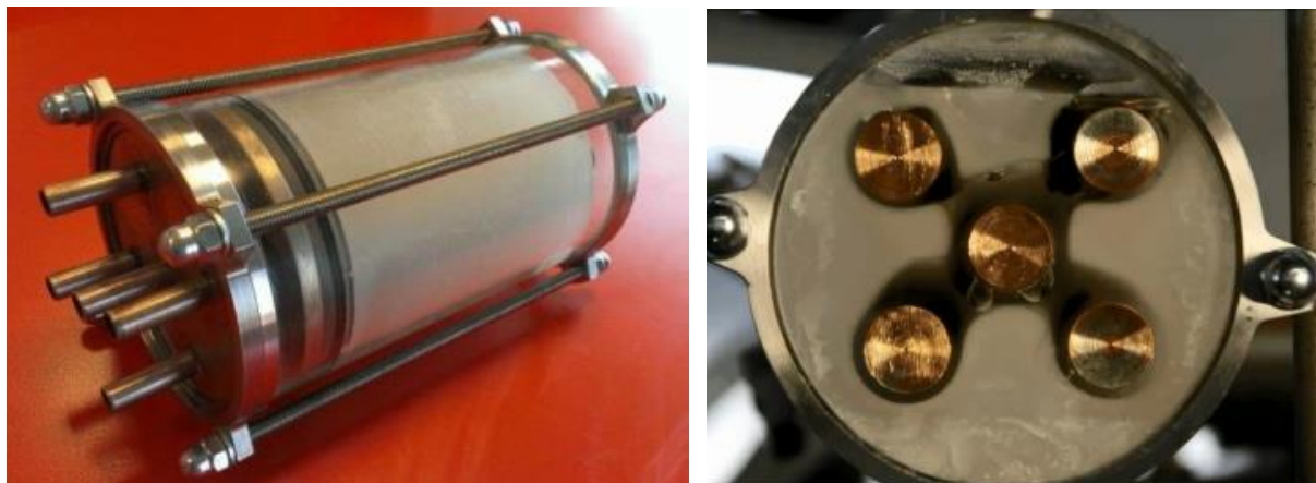
Figure 3: Small scale transparent prototype (a) side view, (b) bottom view, showing the progressing melting front around the tubes.
