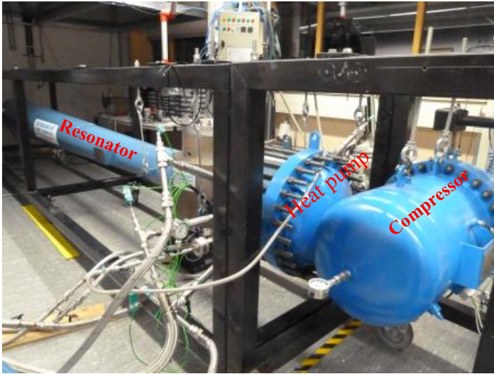
Figure 8 Picture of the thermoacoustic heat pump
