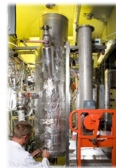
Figure 2: 5 kW th BFB facility at ECN.
