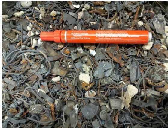
Figure 11: Small pieces of metal, sieved out of bottom ash
