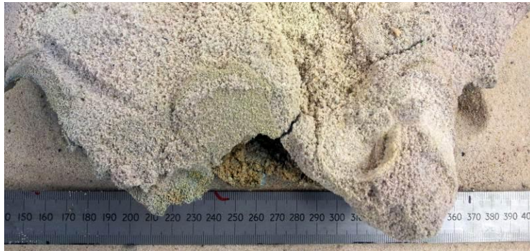
Figure 10: Agglomerate found in Bubbling Fluidized Bed (BFB)
