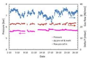
Figure 2. Pressure in, pressure drop over and total gas flow through prereformer and two methanation reactors during 500 hrs test.
