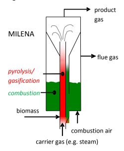
Figure 1. MILENA indirect gasifier with gasification reactor surrounded by combustion reactor.
