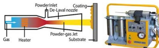
**Figure 1:** Schematic view of cold spray technology (left) and the used equipment, Dymet 423 (right)
