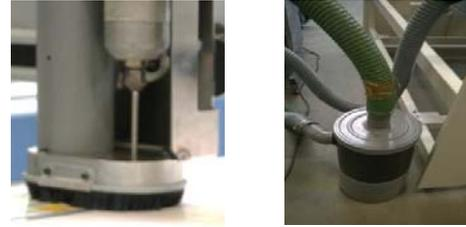
**Figure 4:** Vacuum system to collect the powder that does not adhere to the foil (left) and the cyclone to separate the powder from the air flow
