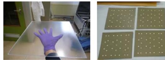
**Figure 11:** Powder coated and pre-heated glass and solar cells (contact areas are cleaned from encapsulant before pre-heating using the contact point cleaner)
