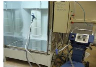
**Figure 6:** Photograph of the used powder coat facility (Norton Encore spray controller and spray booth)
