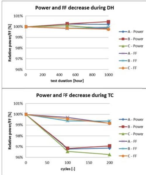
**Figure 8:** Change of power and fill factor during testing modules under DH (left) and TC (right) conditions
