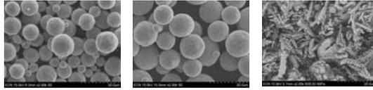
**Figure 2:** Used powders from left to right: spherical 10 micron (A), spherical 20 micron (B) and dendrite <25 micron (C)
