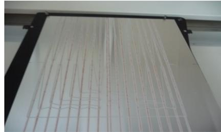
**Figure 5:** 18 lines of copper cold spray corresponding with the position of the front and back contacts
