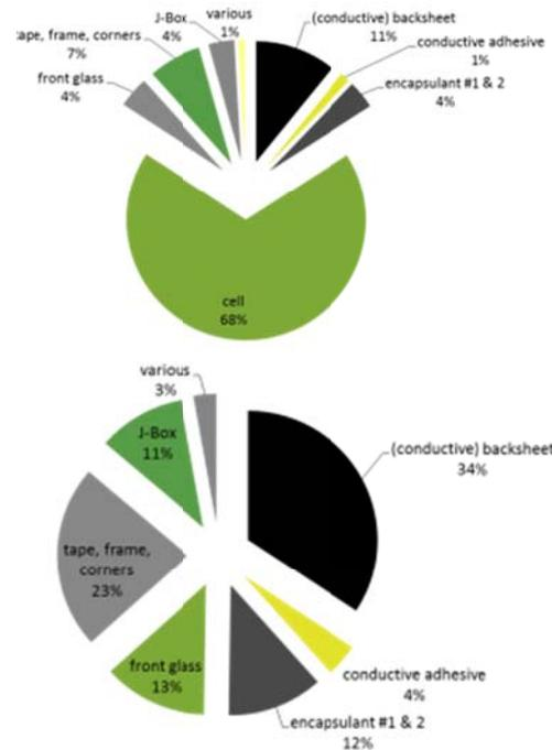
**Figure 15:** Build-up module cost (upper figure) and the contribution of the several module material costs (lower figure)
