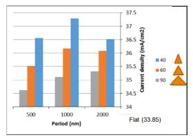
**Figure 4:** Enhancement of  $J_{sc}$  for 2000 nm absorbers through triangular textures with different top angles and periods.
