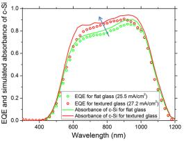
**Figure 5**: EQE of the c-Si bottom cell of a hybrid tandem, for which the front glass was flat (green) or coated with an AR texture (red)
