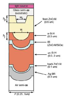
**Figure 2:** Schematic lay-out of a thin-film silicon tandem solar cell on a regular grating. The grating is characterized by the width, w0, and the height, h0, of the trapezoid. A leveling parameter, not shown here, indicates the degree of leveling of the layers deposited on top of this grating.
