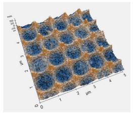
**Figure 6:** 2D periodic texture imprinted in a UV curable lacquer, after annealing at 550  $^{\circ}$ C. The  $R_{pv}$  is about 80 nm; i.e. about 50% of the  $R_{pv}$  of the master.
