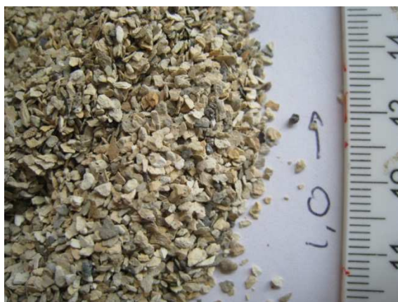
Fig. 5: Bottom ash, sieved > 1mm.
